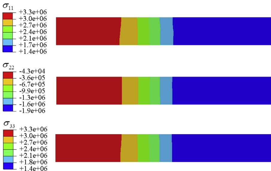
Fig. 9. Stress distribution inside the membrane obtained using the CCM model at the dried state after fast unloading (unit: Pa. Not to scale.).
