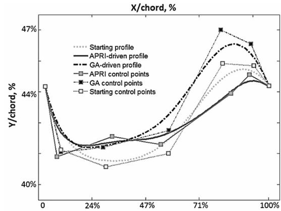
Fig. 4. Airfoil's PS profile and its design variables before and after aerodynamic shape optimization using APRI.
