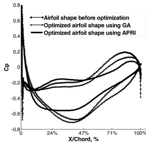
Fig. 6. Comparison of pressure distribution.
