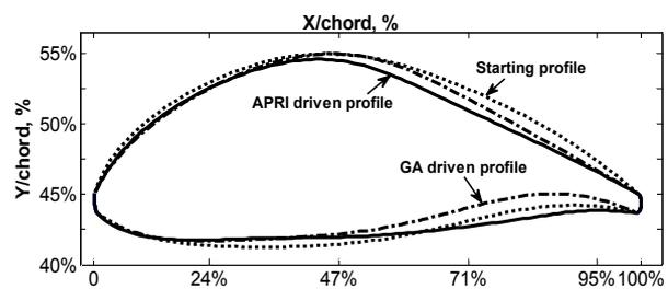
Fig. 5. Whole airfoil profile before and after optimization.
