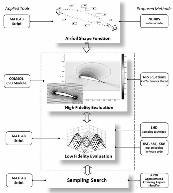
Fig. 1. Integration of tools and methods in airfoil shape optimization.
