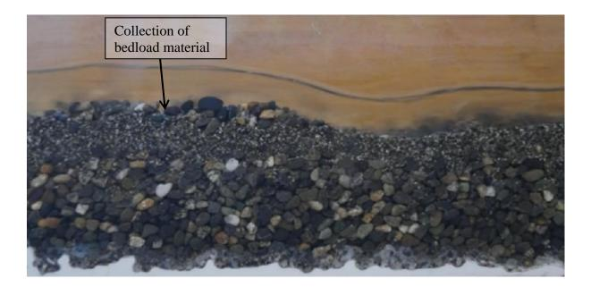
Figure 5.6 Image from the SLR camera of the undulations in the bed surface during the SFU<sub>nat</sub> Experiment S.17 ( $D_f$  =0.6 mm, fine feed/total feed = 42 %). Flow from left to right.
