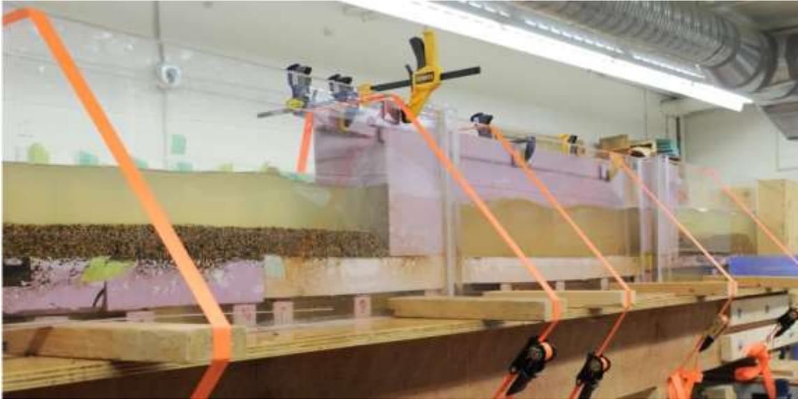
**Figure A1.** Photograph of the flume setup during one of the runs. Entrance and exit reaches are alluviated, while the canyon reach is mostly clear.
