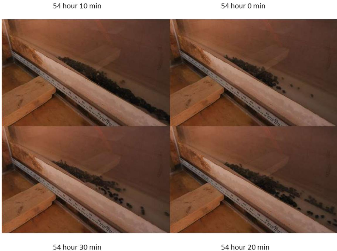
**Figure C1.** Consecutive photographs during Run 5 showing short-term alluviation pattern in the canyon reach. The photos are examples of different stages during an alluviation cycle, and not a sequence of one cycle.
