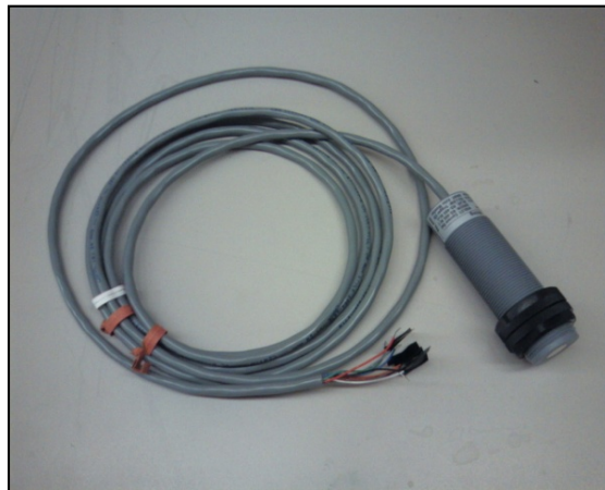
Figure 3-5. A Massa® ultrasonic sensor (Photo taken by author).
