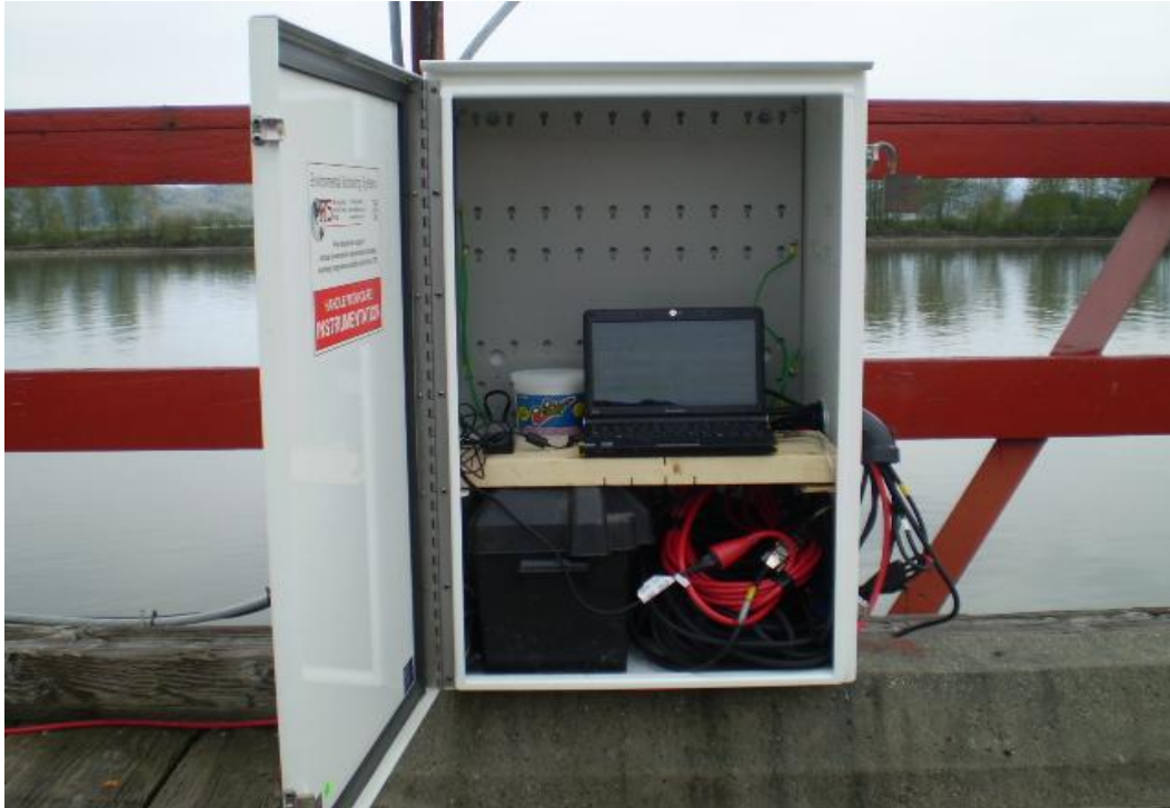
Figure 30: Work station for aDcp housing the computer controlling the instrument and logging data.
