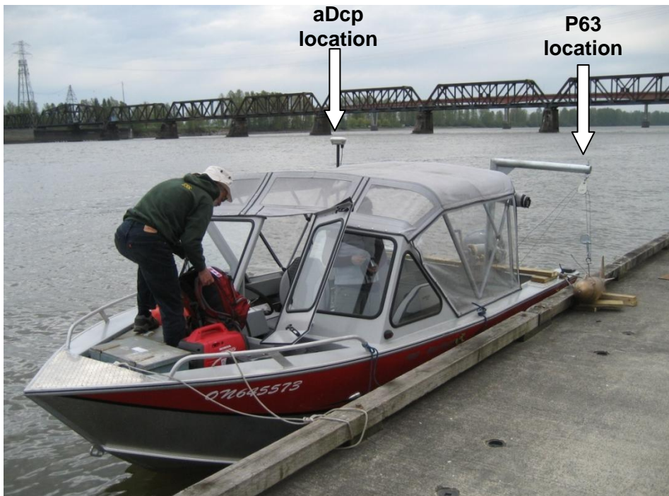
Figure 9: The 19-ft aluminium launch from which the P63 sampler and downward facing aDcp were deployed.
