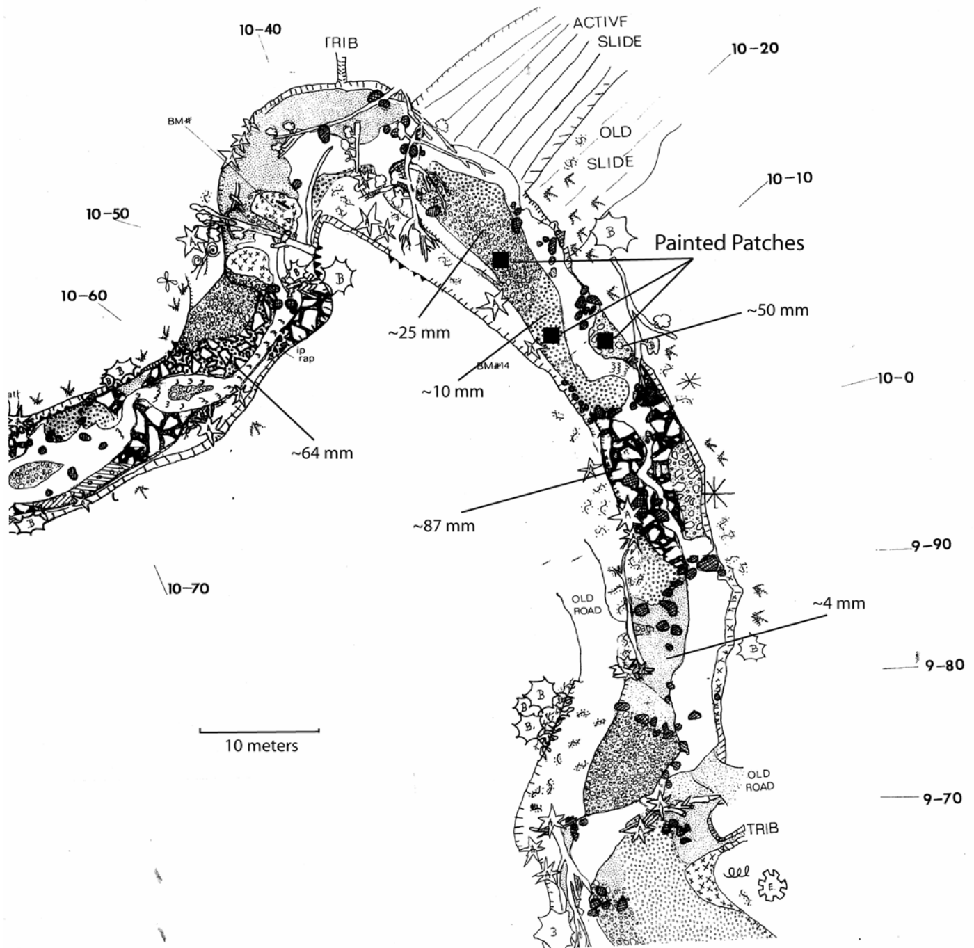
Figure 1. Facies map of Wildcat Creek, near Berkeley, CA, showing locations used in the painted rock study. Numbers along border are distances in meters. Tree locations along the bank are indicated by various symbols. Large woody debris is shown roughly to scale. Average median grain sizes are indicated for each facies type, and area with no pattern was covered by water. Flow is from left to right.
