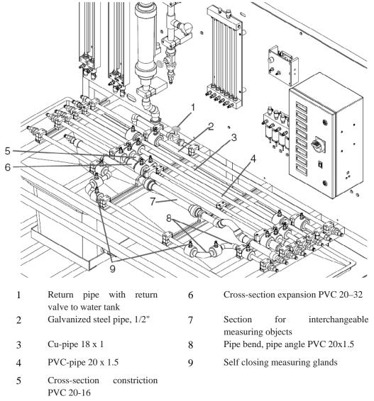
Figure 2- View of the setup test section.
