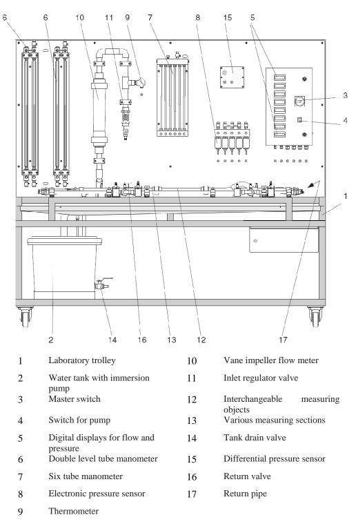
Figure 1- Components of experimental apparatus.
