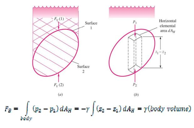
• The line of action of the buoyant force passes through the center of volume of the displaced body; i.e., the center of mass is computed as if it had uniform density. The point which  $F_B$  acts is called the *center of buoyancy*.
