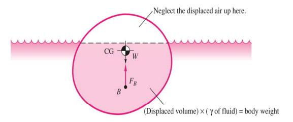
$F_E = \gamma(dtsplaced\ volume) = weight\ of\ the\ floating\ body$
