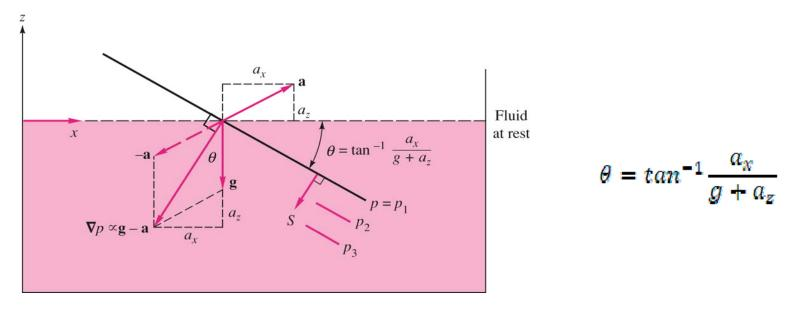
The rate of increase of pressure in the direction g – a is greater than in ordinary hydrostatics
