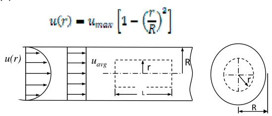
where  $u_{max}$  is the maximum fluid velocity at the center of the tube. Using the definition of the mass flow rate and the concept of average velocity, show that
