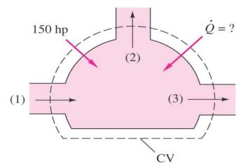
Work is provided to the machine at the rate of 150 hp. Find the pressure p3 in lbf/in<sup>2</sup> absolute and heat transfer in Btu/s. Assume air is a perfect gas with R=1716 and  $c_p = 6003$  ft. lbf/(slug.R).
