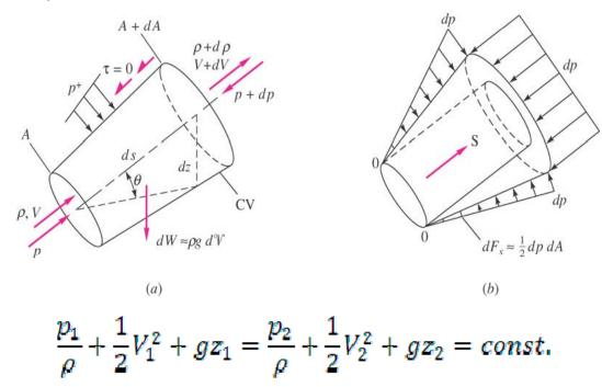
The Bernoulli for <u>steady frictionless incompressible flow along a streamline.</u>
