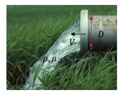
flows through a 25-mm-diameter pipe with a velocity of  $2.6 \, m/s$ . Determine the value of the Reynolds number using (a) SI units, and (b) BG units.
