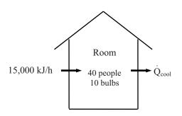
**3-51** The lighting energy consumption of a storage room is to be reduced by installing motion sensors. The amount of energy and money that will be saved as well as the simple payback period are to be determined.
