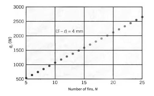
The foregoing calculations are based on the assumption that h is not affected by a reduction in the fin gap. The assumption is reasonable as long as there is no interaction between boundary layers that develop on the opposing surfaces of adjoining fins. Note that, since  $NA_f \gg 2\pi r_l(H - N_t)$  for the prescribed conditions,  $q_t$  increases linearly with increasing N.
