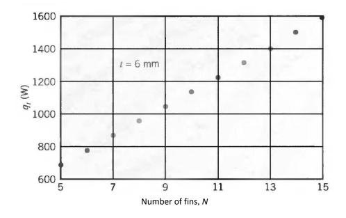
The number of fins could also be increased by reducing the fin thickness. If the fin gap is fixed at (S - t) = 4 mm and manufacturing constraints dictate a minimum allowable fin thickness of 2 mm, up to N = 25 fins may be accommodated. In this case the parametric calculations yield
