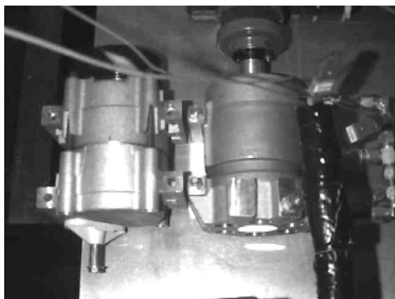
Fig. 31. A 155 cm 3 R-134a compressor (left) next to a 21 cm 3 CO 2 compressor (right) [91].
