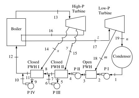
*Analysis* The compression processes in the pumps and the expansion processes in the turbines are isentropic. Also, the state of water at the inlet of pumps is saturated liquid. Then, from the steam tables (Tables A-4, A-5, and A-6),
