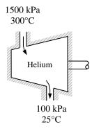
There is only one inlet and one exit, and thus  $\dot{m}_1 = \dot{m}_2 = \dot{m}$ . We take the turbine as the system, which is a control volume since mass crosses the boundary. The energy balance for this steady-flow system can be expressed in the rate form as
