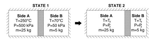
Step 1: Draw a diagram to represent the system showing control mass/volume of interest.
