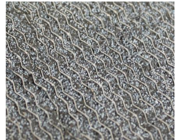
Sorbent on heat exchangers for sorption chiller tests: ZO 2 coating, ZO 2 pellets, empty heat exchanger and CaCl 2 composite
