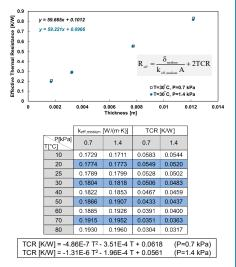
Thermal contact resistance compared to the resistance of medium is significant and should be considered in adsorption studies.
