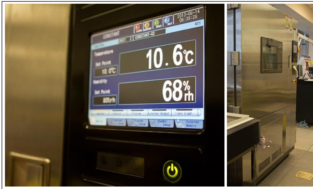
Figure B2. ESPEC environmental chamber used for emissivity measurement tests
