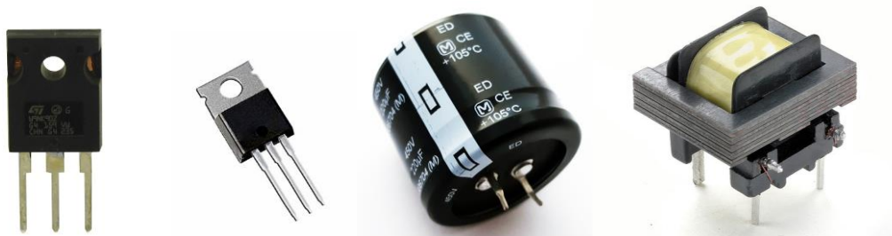
Fig. 3: Power electronic devices: Left: TO-247 MOSFET; Left middle: TO-220 diode array; Right middle: electrolytic capacitor and Right: transformer
