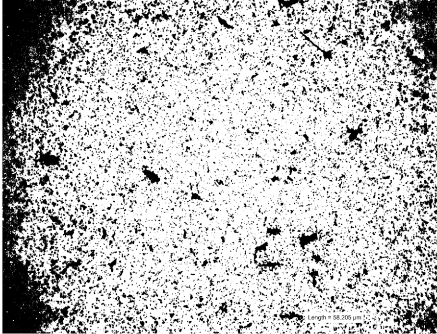
Fig. 26: Binary of optical image of aluminum oxide at 20x magnification
