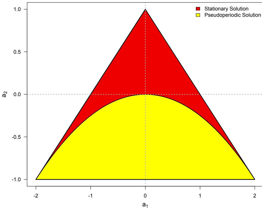
Figure 4.1: Parameter plane for the solution space of a set of movement parameters a_1 and a_2 that solve a set of stationary AR(2) difference equations.
