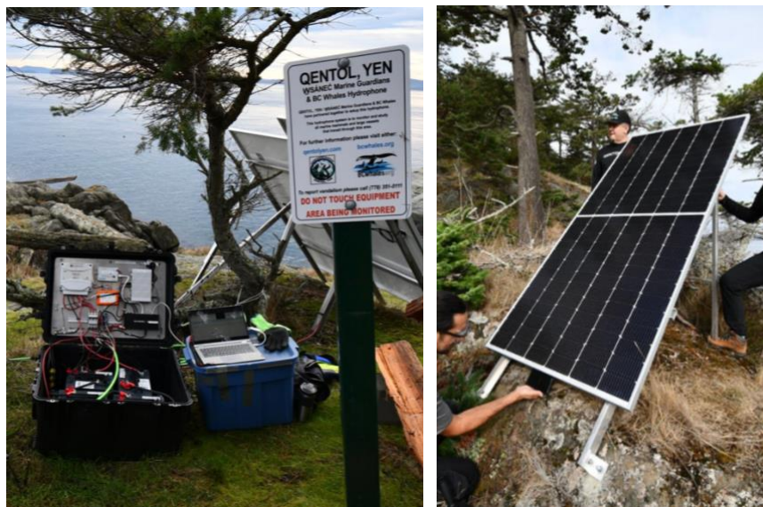
Figure 2. Photograph of the hydrophone deployment setup. Left: Monitoring system (black box) containing computer, battery; Right: Solar panel.
