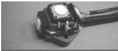
Figure 2: Polhemus sensor with attached buttons.
