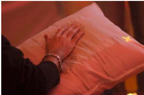
Figure 2. Pillow with actuators touchpad, LED display and vibrator.
