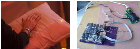
Figure 1: Pillow with actuators touchpad, LED display and vibrator (photos by courtesy of Jan Sprij)
