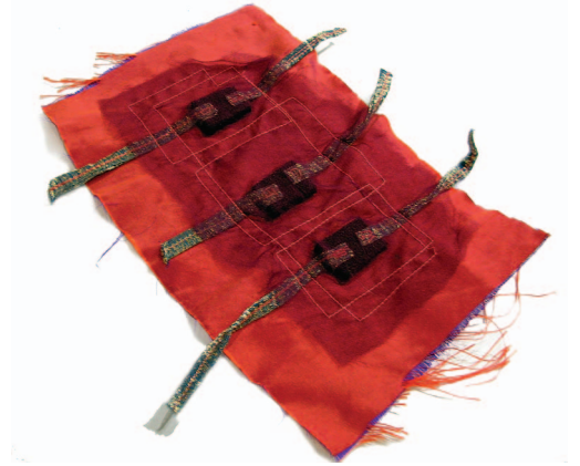
Figure 1. Example of how sensors and conductive fabrics (soft cables) become constructive elements of garments.
