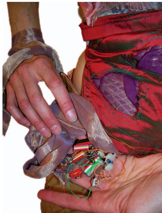
Figure 2. Sensor and actuator electronics embedded within fabric enable explorations in garments as physically expressive devices.
