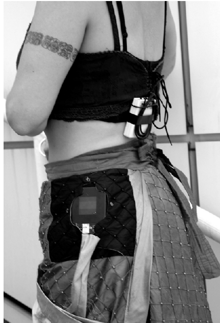
Figure 2: Exhale breathband measures breath, while RFID tag enables breath exchange.
