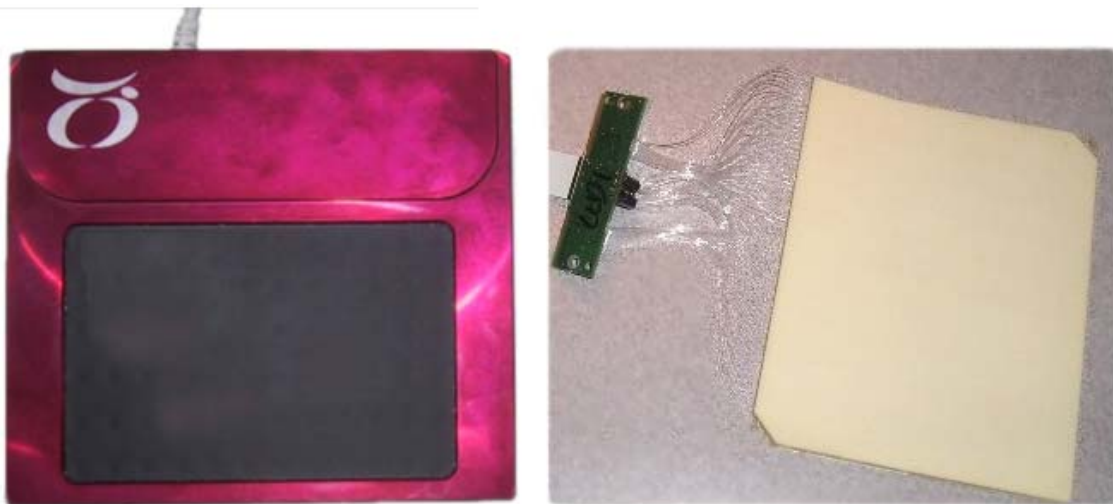
Figure 76. Tactex Multitouch Controller with Embedded 72 Taxel Optical Fibre Array (2001)
