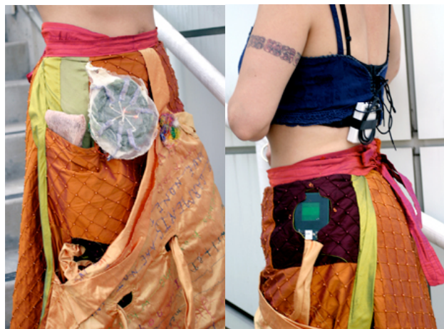
Figure 7. exhale skirt with LED array and RFID
