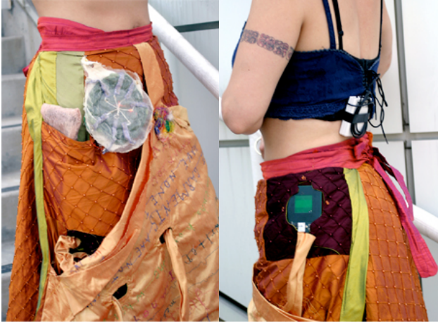
Figure 8 exhale skirt with LED array and RFID
