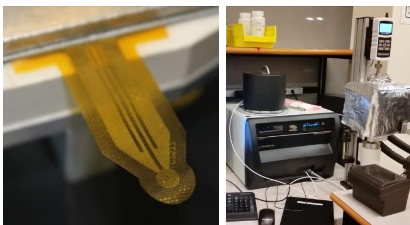
Transient plane source (TPS) thermal constants analyzer with "hot disk" nickel wire sensor and environmental chamber
