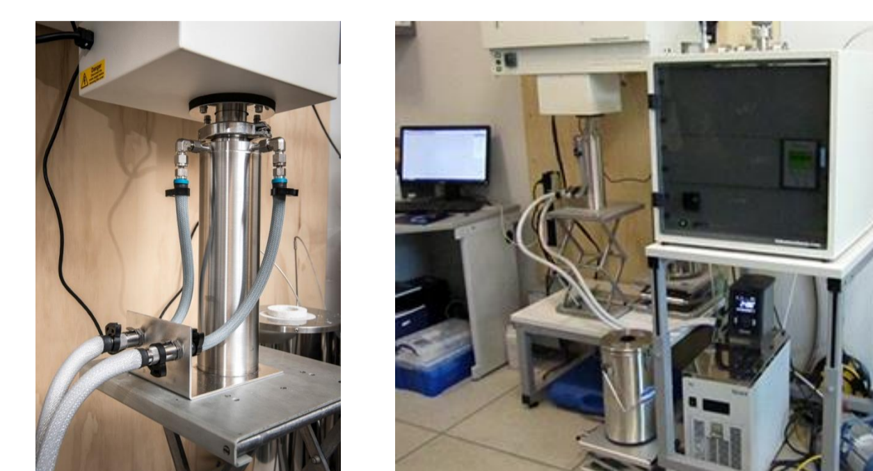
Thermogravimetric vapor sorption analyzer
