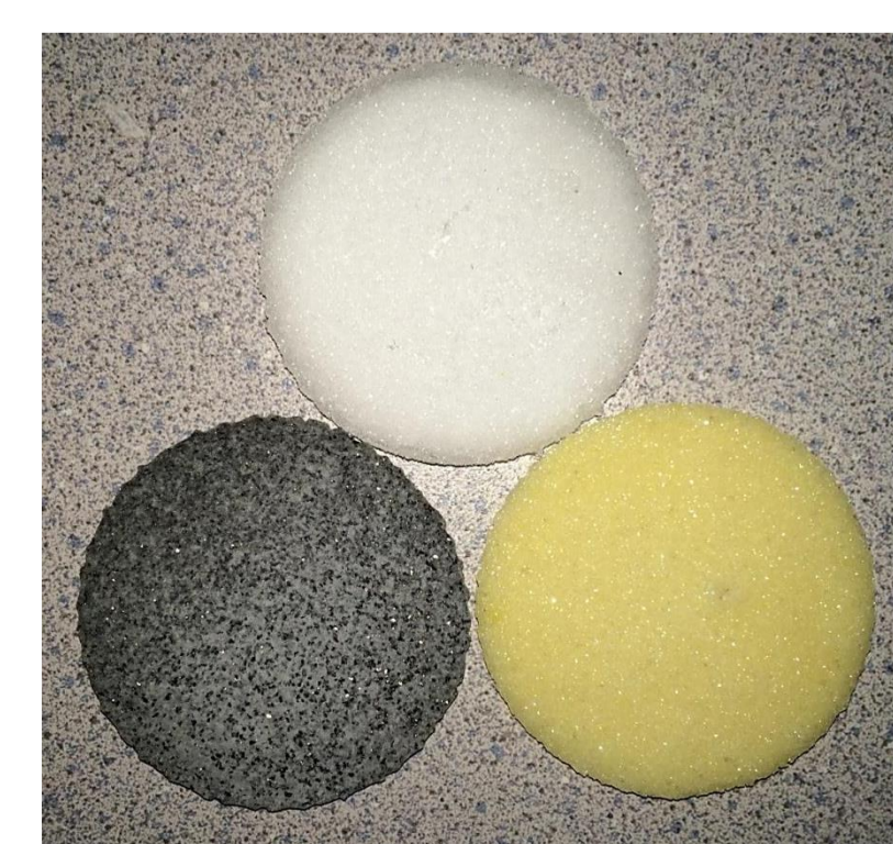
Composites containing silica gel organic binder and graphite flake
