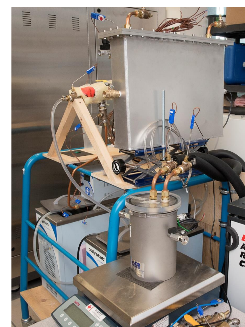
Adsorption cooling system lab-scale prototype
