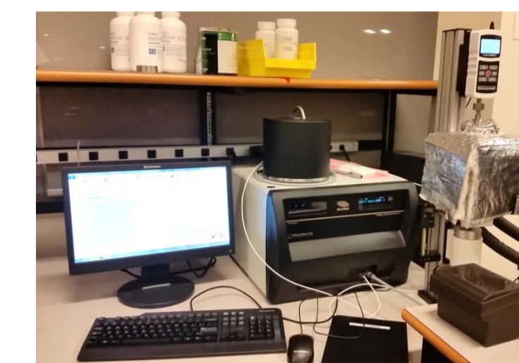
Transient plane source (TPS) thermal properties analyzer
