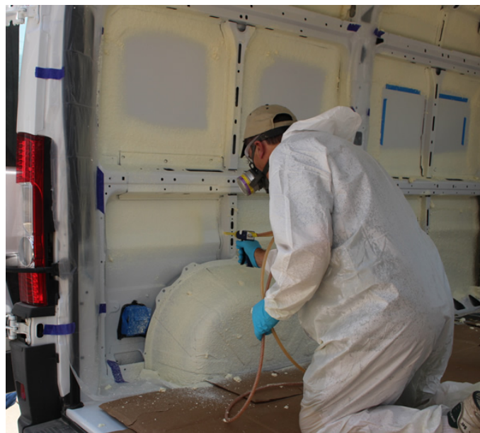
Figure 1.3. Spraying Polyurethane foam on the interior walls of a reefer van [61]
