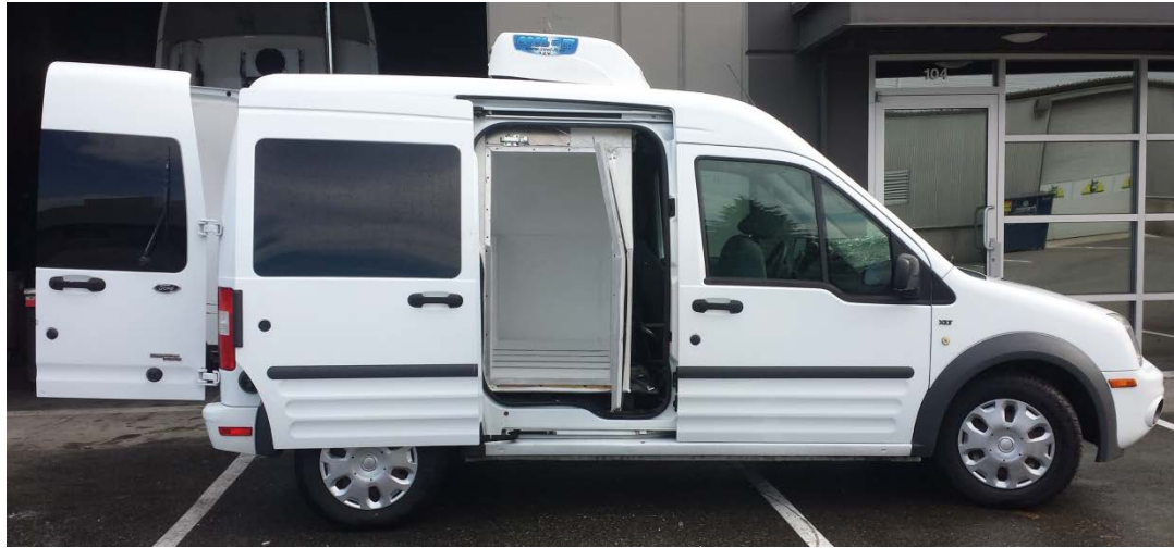
Figure 4.21. Side view of the insulated van after installation of the electric refrigeration system
