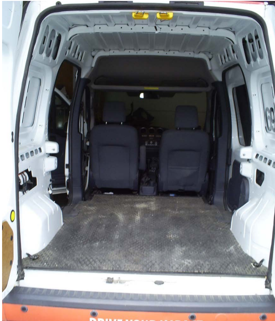
Figure 4.3. Interior view of the Ford Transit Connect, which is to be insulated for reefer applications
