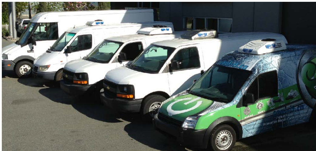
Figure 1.2. Commercial reefer vans that are the subject of this project
