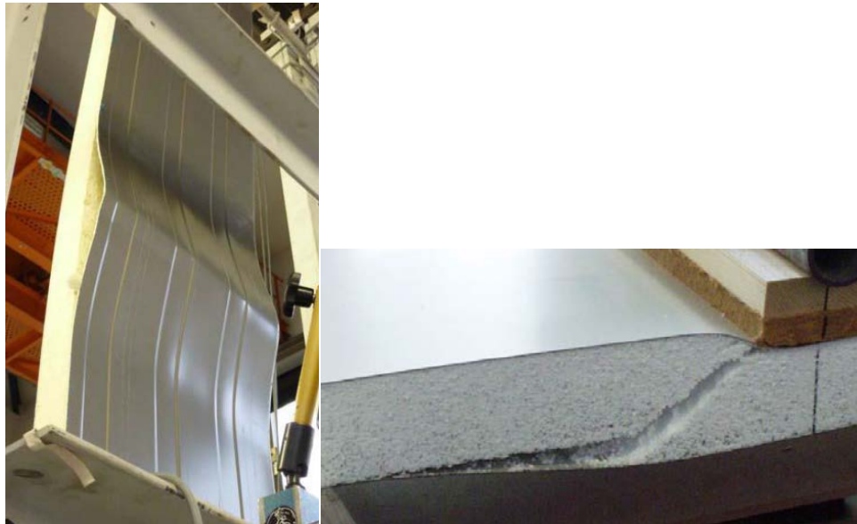
Figure 2.19. Left: buckling of the compressed face. Right: Shear failure of the core [46]
