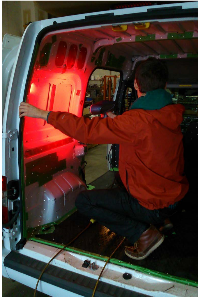
Figure 4.5. Taking the 3-D image of the vehicle interior surface using a HANDYSCAN scanner
