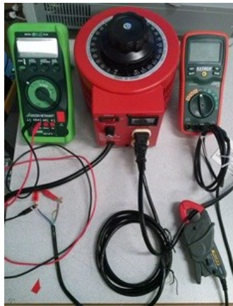
Figure 2.3. Power supply measurement: SC-20MVariac (middle) and Extech 430 multimeters (two sides)
