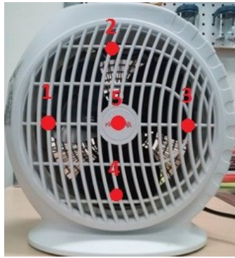
Figure 2.5. Five random velocity measurement points on the fan surface
