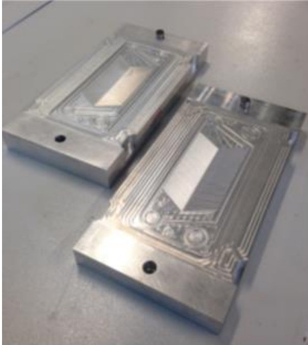
Figure 37. Dies for fabrication of optimized chevron-type graphite plate heat exchanger.
