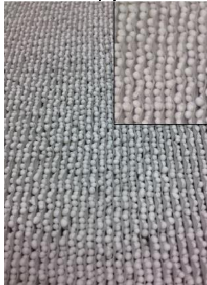
Figure 4-3 The actual heat exchanger used as adsorber bed
