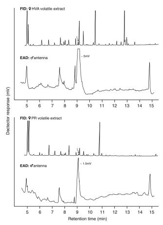
**Fig. 4** Flame ionization detector (FID) and electroantennographic detector (EAD: male *Timema cristinae* antenna) responses to effluvium volatiles from female HVA (*top*) and female PR (*bottom*). Chromatography: DB-5 GC column (0.32 mm ID × 30 m); temperature program: 50°C (1 min), 10°C per min to 200°C, then 25°C per min to 280°C. Most antennally active compound marked by an arrow
