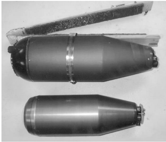
Fig. 1. Hi-8 (top) and digital video (bottom) Crittercam units. A dorsal fin clamp used to attach Crittercams is attached to the Hi-8 unit. Clamps are lined with coarse sandpaper to grip the shark's fin, but do not cause tissue damage or leave any noticeable marks on the dorsal fin
