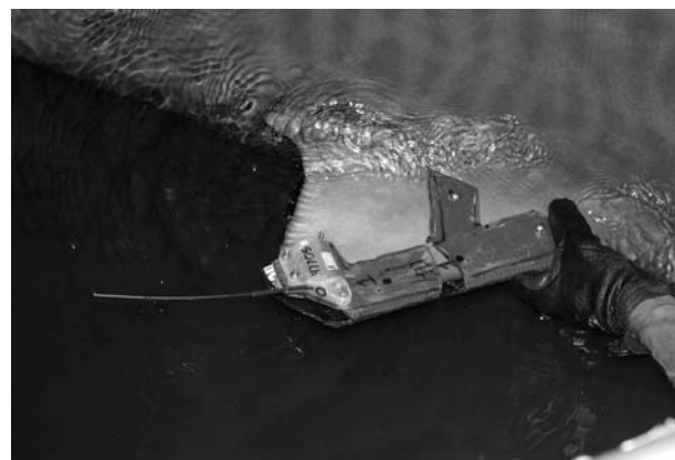
Fig. 1 SPOT4 tag attached to a tiger shark in Shark Bay. Note that the saltwater switch and antenna are positioned above the dorsal fin to maximize the probability that the tag will transmit when the shark is near the surface
