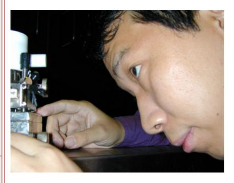
SFU materials chemist Hogan Yu points to the sample stage of an atomic force microscope. The microscope provides pictures of atoms on or in surfaces placed on the stage.
