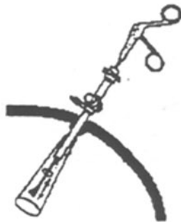
Figure 1. Degrees of freedom (DOF) of a conventional instrument in endoscopic surgery (from Melzer et al., 1992, p.15). Excluding the end-effectors, there are 4 DOF: 1) translation along the shaft of the tool, 2) rotation around the translational axis, 3 & 4) limited incline of the shaft pivoted in the abdominal wall.
