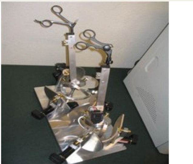
Figure 1: An embodiment of the invention, showing a two-handed operation system with eight haptic degrees of freedom.
