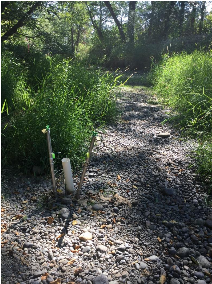
Figure 1: Bertrand Creek at Otter Park in the Bertrand Creek Watershed. Photograph taken August 8, 2018 when the stream was almost dry. Shown in the foreground are nested instream piezometers (steel tubes), along with a white section of pipe used to shield two Onset Tidbit temperature loggers placed at two depths in the streambed.
