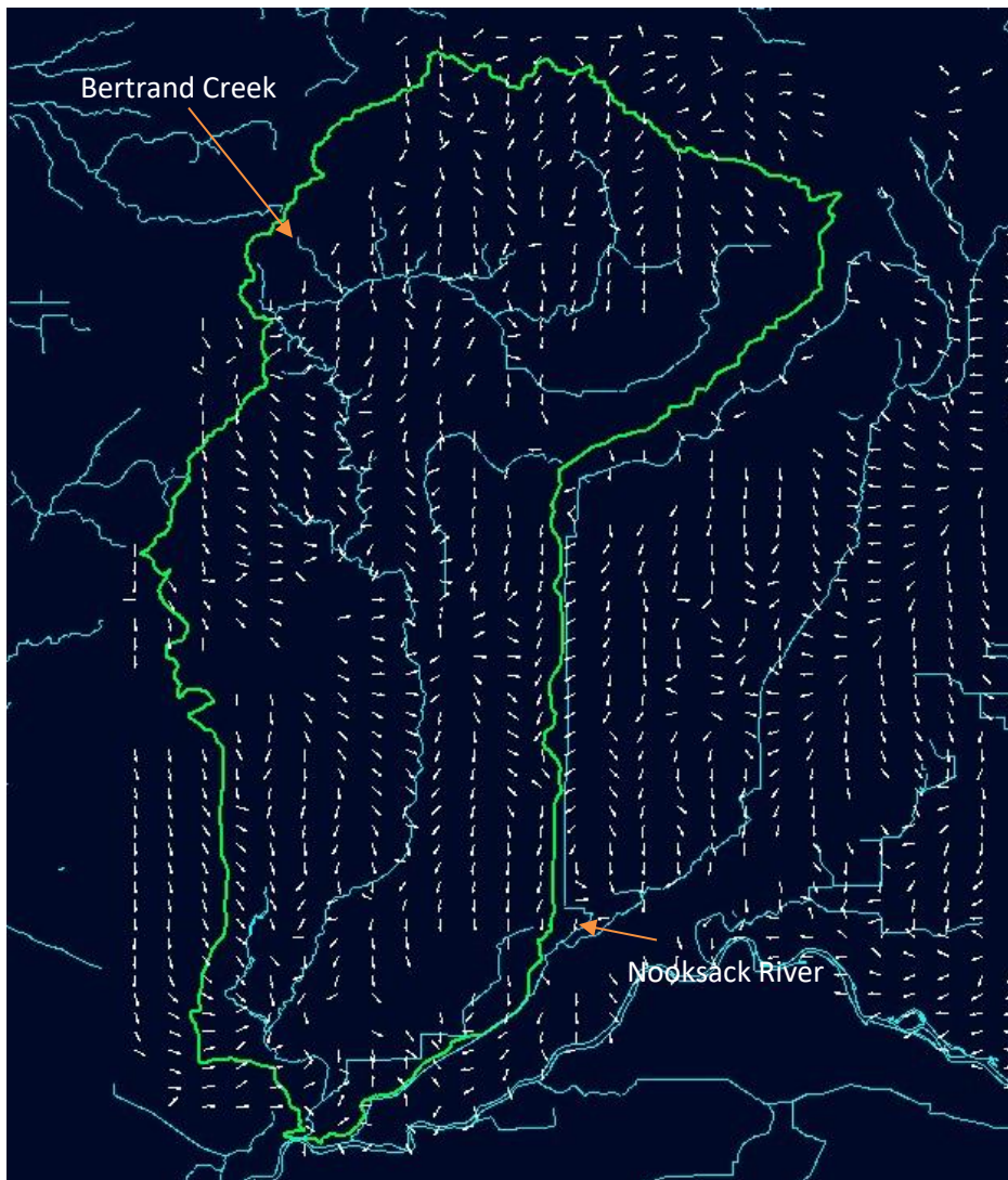
Figure 15: Velocity field map showing the direction of groundwater flow through the Bertrand Creek Watershed in the uppermost layers of the model in the original Abbotsford-Sumas model.
