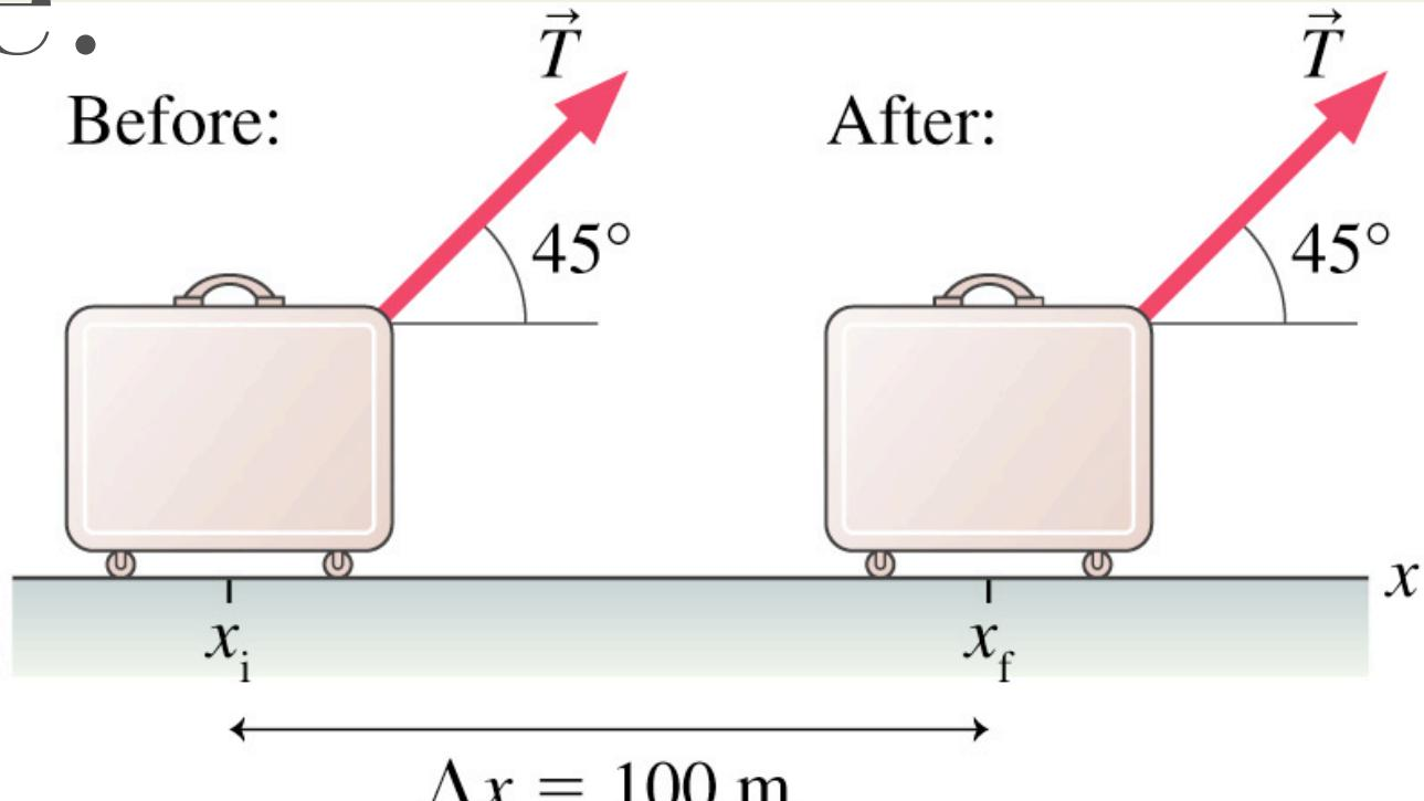
$$\begin{aligned}W &= T\Delta x \cos \theta \\&= (20 \text{ N})(100 \text{ m})\cos 45^\circ \\&= 1410 \text{ J}\end{aligned}$$
