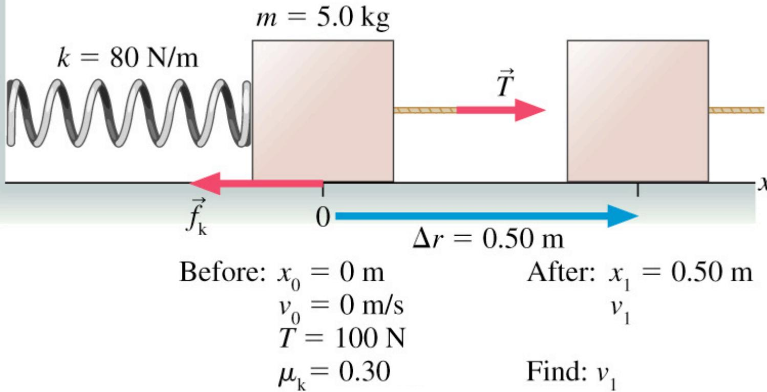
Rope pulls box tied to the wall with a spring.
