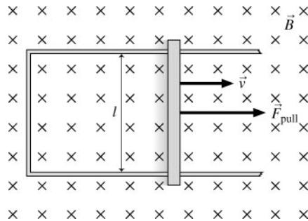
The wire is pulled with a constant force in a magnetic field. This results in a motional emf and produces a current in the circuit. From energy conservation, the mechanical power provided by the puller must appear as electrical power in the circuit.
