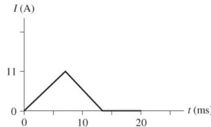
(b) The maximum current of 11 A occurs when the flux is changing the fastest and this occurs when the loop is halfway into the region of the field.
