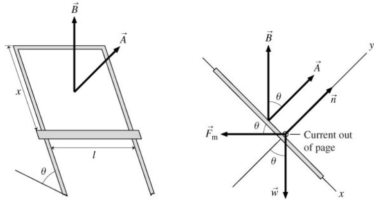
The moving wire creates a changing area and corresponding change in flux. This produces an induced emf and induced current. The flux through the loop depends on the size and orientation of the loop.
