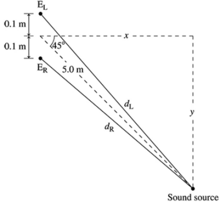
We know the speed of sound in room-temperature air is 343m/s. So, all we need is to calculate the path difference between the waves traveling to the left and right ears. OK, so what is the distance from the source to the left ear ( $E_L$ )?
