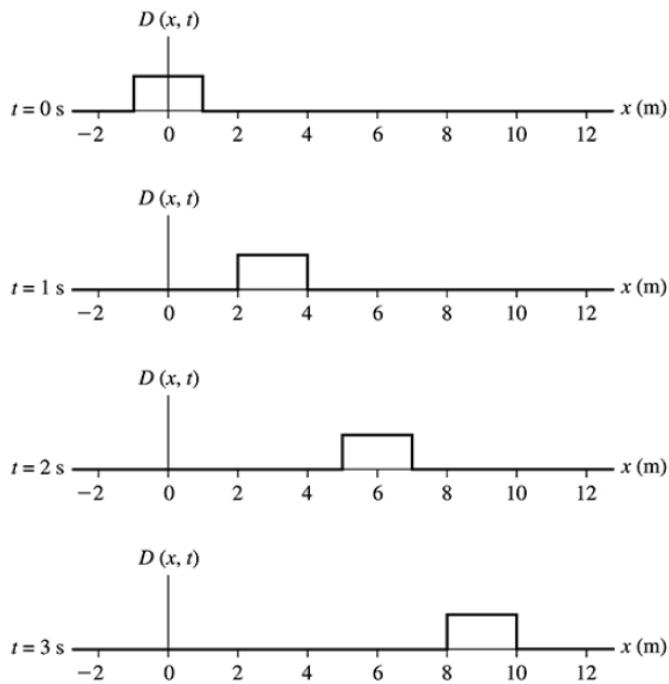
b) The leading edge of the pulse moves forward 3m each second. Thus, the wave speed is 3m/s.
