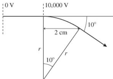
The electron is deflected by  $10^\circ$  after moving along a circular arc of angular width  $10^\circ$ .
