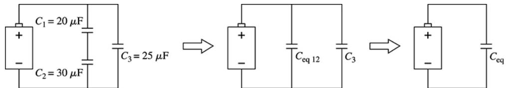
The pictorial representation shows how to find the equivalent capacitance of the three capacitors shown in the figure.
