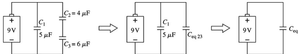
The pictorial representation shows how to find the equivalent capacitance of the three capacitors shown in the figure.
