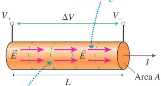
Equipotential surfaces are perpendicular to the electric field.
