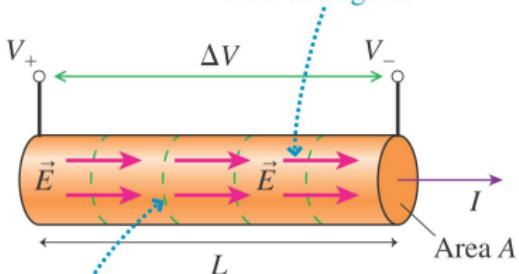
Equipotential surfaces are perpendicular to the electric field.
