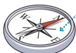
The needle of a compass is a small magnet.
