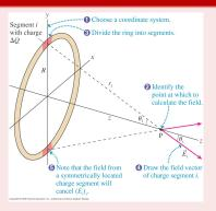
A thin ring of radius R is uniformly charged with total charge Q. Find the electric field at a point on the axis of the ring.
