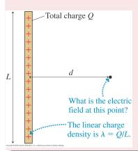
Find the electric field strength at a distance d in the plane that bisects a rod of length L and total charge q.
