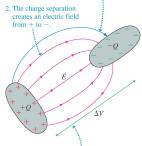
Because of the electric field, there's a potential difference between the electrodes.
