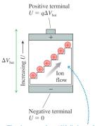
The charge escalator "lifts" charge from the negative side to the positive side. Charge q gains energy  $\Delta U = q \Delta V_{\rm bat}$ .
